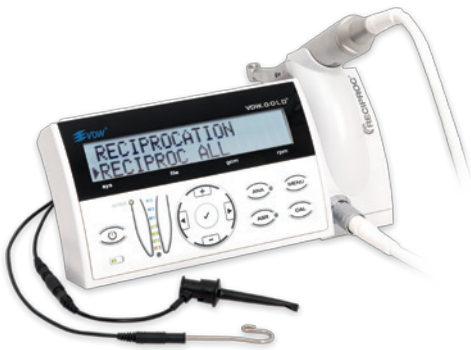
VDW.GOLD®RECIPROC® with integrated apex locator
